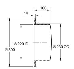
holes orientated as shown in relation to top surface of the enclosure. Ø14mm x 16 holes Α equi-spaced on  $\phi$  262.0 PCD ±1 11.25° IDØ 220 ±1 -0 ø ODØ300 ±1 Ø *`*ø ¢ ¢ Ļ ¢ C ¢- ¢-Ø
