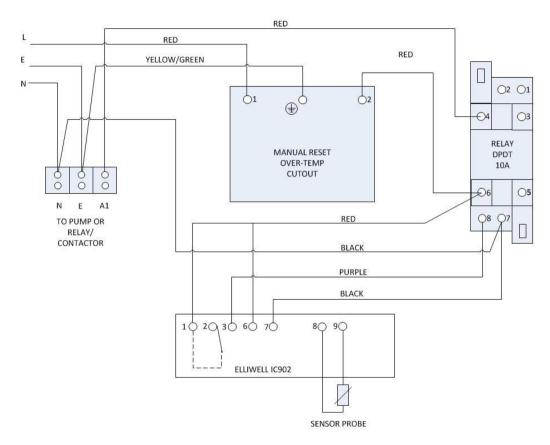
Wiring Diagram – Pump/C Controller
