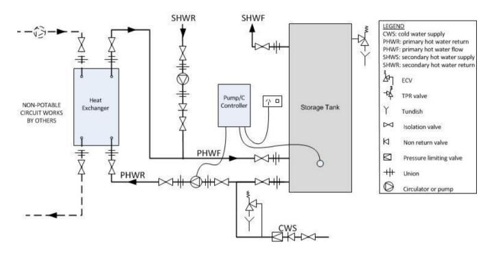
Typical Installation 1 x Heat Exchanger and Storage Tank
