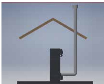
Room Sourced Vertical Flueing
