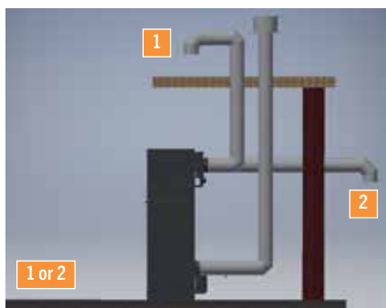
Room Sealed Vertical Flueing
