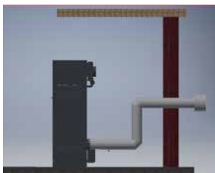
Room Sourced Horizontal Through-the-Wall Flueing
